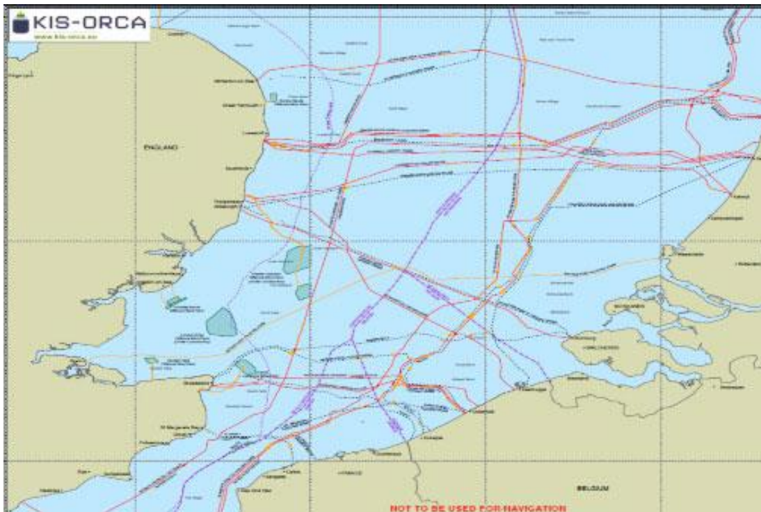
Figure no. 4. Chart showing all cable inter-connectors, export cables and telecommunications cables (ESCA, 2024)
